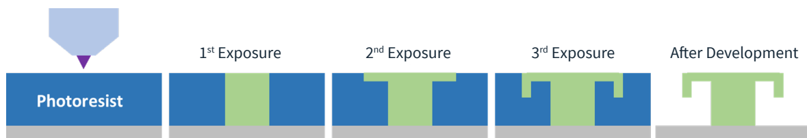
Figure 1: Illustration of the multilayer exposure process used to create 3D structures via grayscale lithography.
